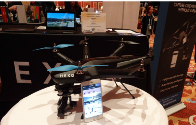
The Hexo is a high performance drone that boasts a 4K camera and the ability to travel at up to 45mph.
