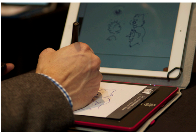
iSketchnote's stylus and pressure sensitive pad enable you to simultaneously draw both a paper and digital image.
