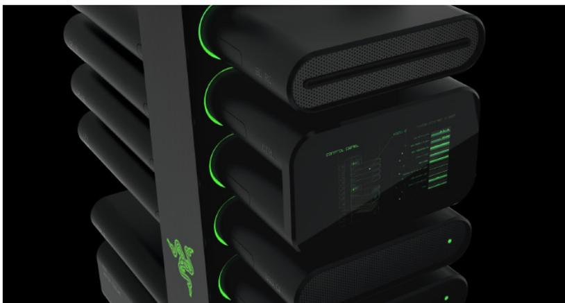
**A**ccording to Razer: "Project Christine is a revolutionary new concept design that allows users to build and customize PCs in any configuration without any prior technical knowledge. Choose any module on-the-fly in any combination, whether it's the CPU, memory, graphics card, storage or power supply module, and simply plug it in. The PCI-Express architecture of Project Christine automatically syncs the components."
